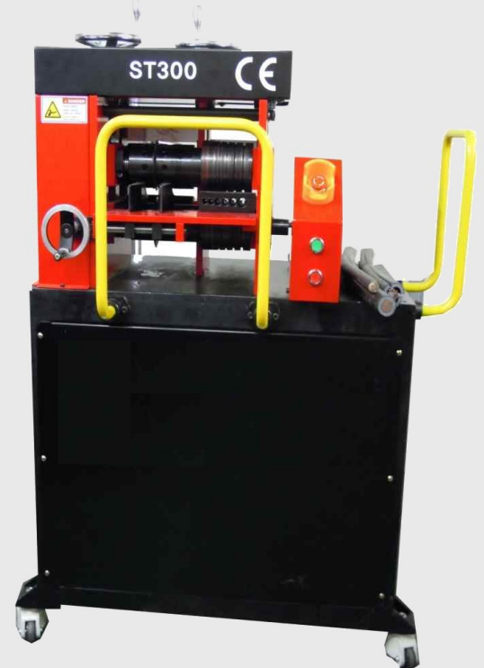
ST300 To strip cable between 1 mm and 60 mm.
